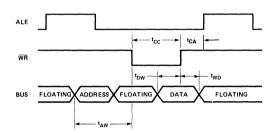
Input and Output Waveforms for A.C. Tests
